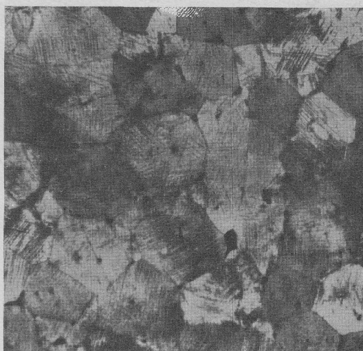
Fig. 4. Showing structures of (a) sand cast and (b) centrifugally cast brass specimen, annealed at 538°C for 1 hour; x 100.
