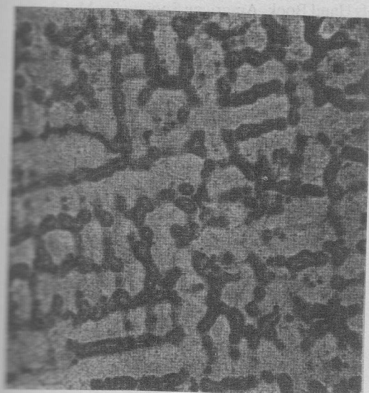
Fig. 4. Showing structures of (a) sand cast and (b) centrifugally cast brass specimen, annealed at 538°C for 1 hour; x 100.
